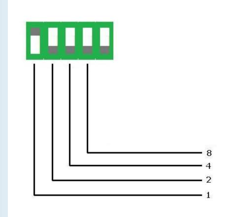
Flipping the switch UP adds the number indicated to the base address. Thus, if the switches marked 1 and 8 were UP, the base address would be 9. The 16 switch is on option switch 2.
