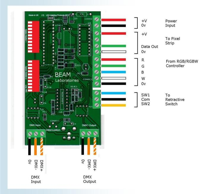
Please note that the PixelatorPlus requires at lease one control input to operate. However, the retractive switch can be used in conjunction with DMX or PWM inputs to offer a simple on/off wall switch override.
